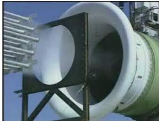
GE90 hail test – similar set up used for sand testing
