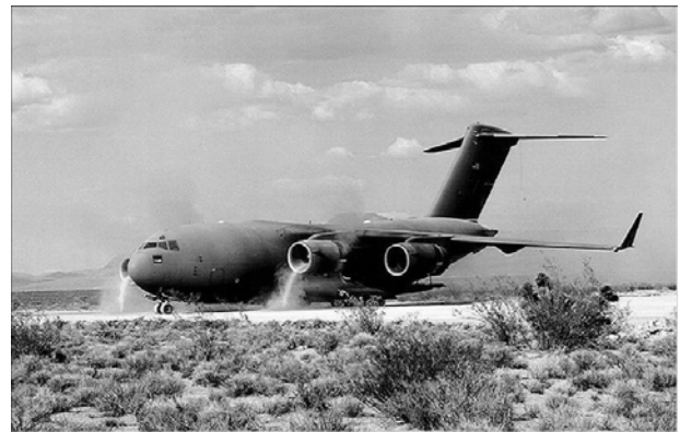
Figure 1. Sand ingested into a C-17 during takeoff.
