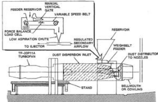
Dunn/Baran/MilatchImages. ASME Large engine research cell, 1996. Operation of Gas Turbine Engines in Volcanic Ash Clouds
