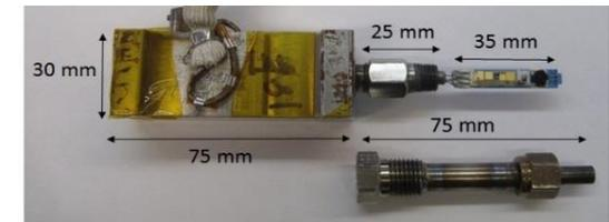
Sensor probe with electronics
