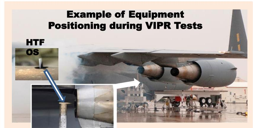
**ESS with HTFOS installed behind the engine exhaust**
