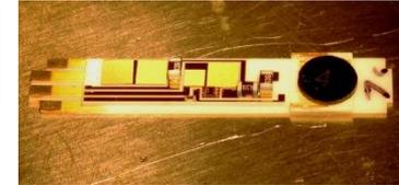
High Temperature Electronics Circuit
